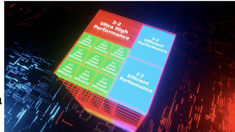
Diagram 2: N3 with FinFlex enables a designer to choose the ideal FIN configuration for each functional block on a chip.
